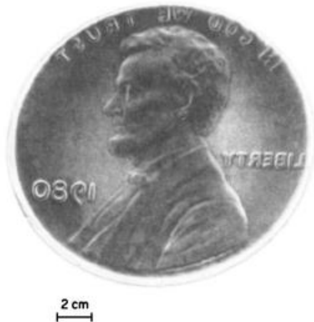
Figure 3 Longitudinal acoustic wave (50 MHz) image at 10 times, of Lincoln's head on the obverse surface of a US penny (courtesy of E. Lynk, General Electric Company).
